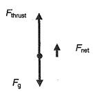
$$F_{\text{net}} = 3,110,000 \text{ N} - \left(232,000 \text{ kg} \times 9.80 \frac{\text{m}}{\text{s}^2}\right)$$
